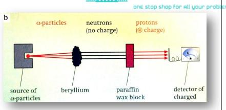
The alpha particles had knocked out neutrons from the beryllium, and in turn these knocked out protons out of the wax.
