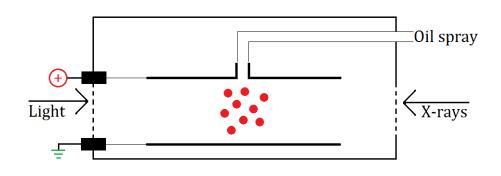
He gave the oil drops negative charge by spraying them into air ionized by Xrays. He adjusted the charge on the plates so that the upward force of attraction equaled the downwards force of gravity, and so the
