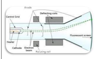
glass causes a shadow. They proposed that the glow was caused by rays coming from the cathode, called <u>cathode rays</u>.
