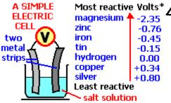
Most reactive Volts\* magnesium ♣-2.35 4. Simple Cells or batteries
