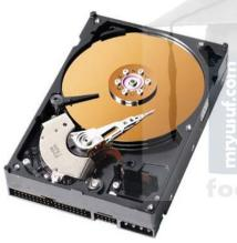
A hard disk drive (HDD), commonly referred to as a hard drive, hard disk, or fixed disk drive, is a non-volatile storage device which stores digitally encoded data on rapidly rotating platters with magnetic surfaces. Strictly speaking, "drive" refers to a device distinct from its medium, such as a tape drive and its tape, or a floppy disk drive and its floppy disk.
